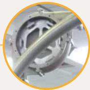
Notched angle gears wheel for discs indexing and setting in motion of the cable
